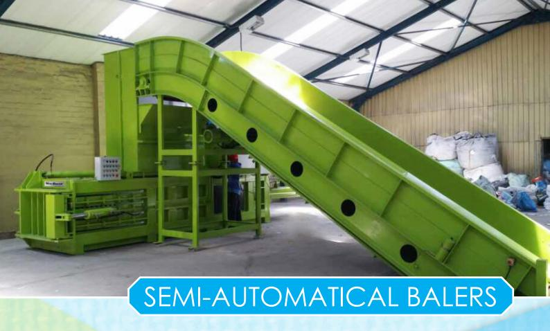
The semi-automatic plastic baler is widely used to compress almost all the loose materials like paper, cardboard, OCC, ONP, books, magazines, plastic bottles, plastic film, textile waste, cans, tins and aluminum scraps etc.
